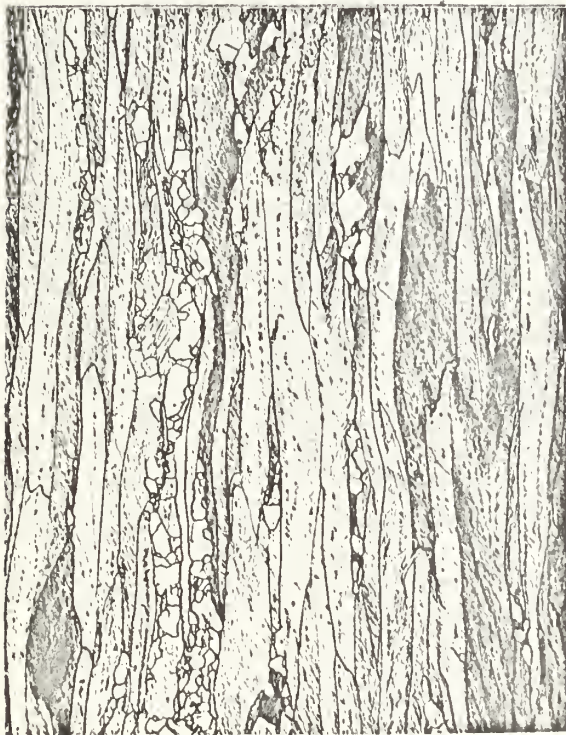
FIG. 7 AT 540°C FOR 6 MINUTES (ROCKWELL 30T 65.9)
